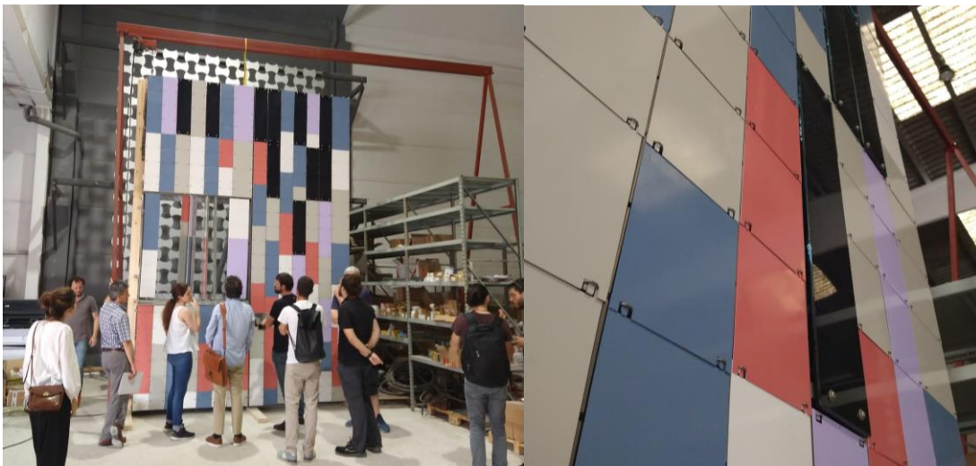
PLURAL pilot project prototype for an AHC residential building in Terrassa, at Denvelops facilities – Ph. Internal archive
